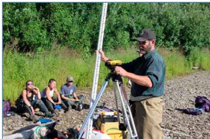
Dan Gillikin shows use of a level to make accurate measurements of the stream bottom along a transect line during the 2017 George River Science Internship. Photo by Dave Cannon.
