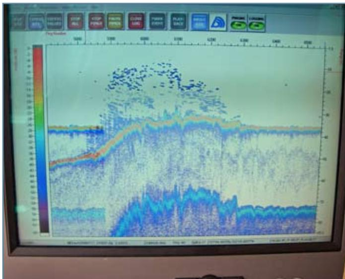
*Screen of the Biosonics DT-X echosounder showing a school of black rockfish associated with a high slope area.*
