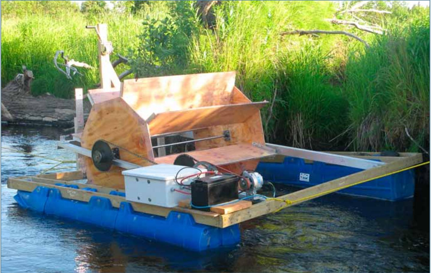
*The prototype paddlewheel hydro-generator produces 2–3 amps/hr at current velocities around 1 m/s. Photo by Mike Parish.*
