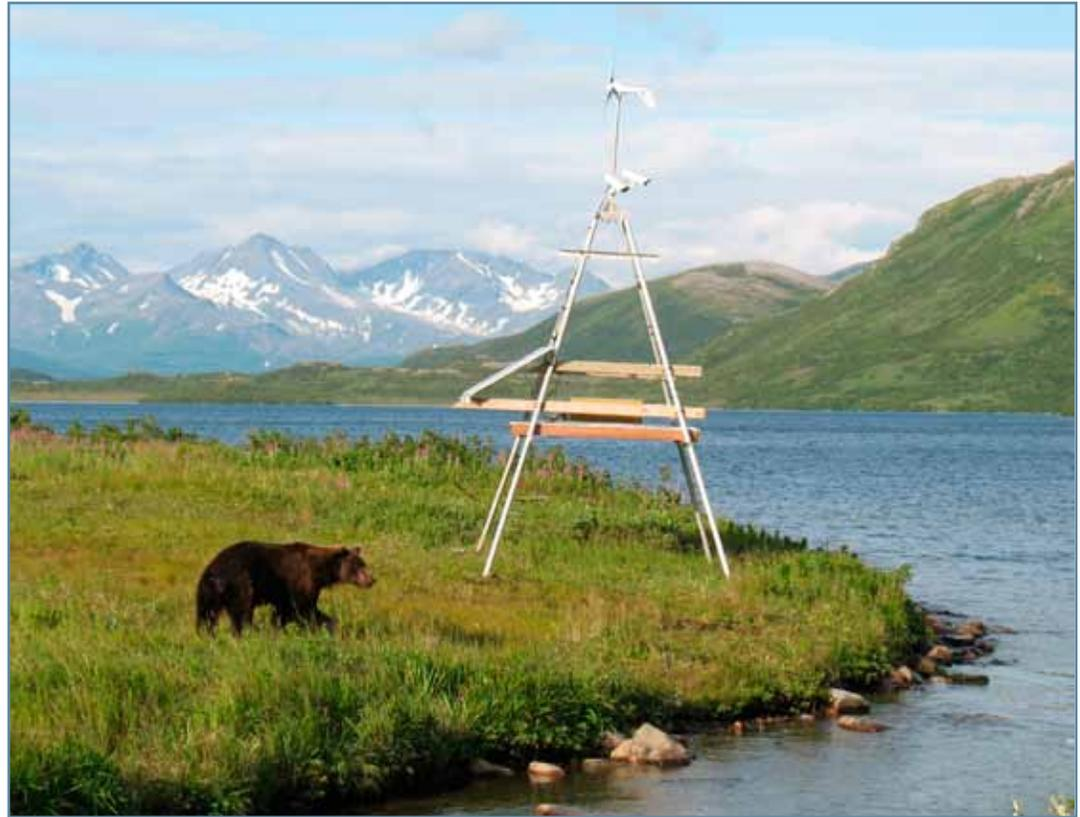
*The AVCT at the outlet of Chenik Lake. All system components are contained on the quadrapod, with sensitive electronics housed in a strongbox on the platform. Photo by Ted Otis.*
