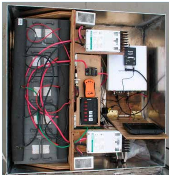
*Electronic components housed inside the aluminum strongbox include: deep-cycle batteries, time-lapse DVR, monitor, fused switch panel, charge controllers and load-dispersion devices. Photo by Ted Otis.*
